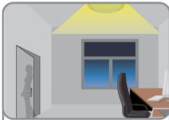
When the room is empty, light dims to stand-by level (10% / 20% / 30%) after the hold-time.
